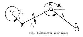
Where  $P_0$  is the initial position,  $d_1$  and  $\theta_1$  are the first path and heading angle. Thereby we can calculate the next position  $P_1$  and so forth.
