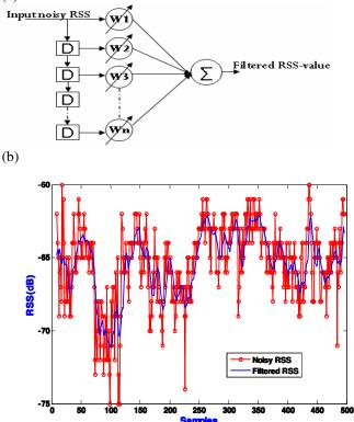
Fig. 2, Time delayed NN for noise reduction (a), Noisy rss at the TDNN input and filtered RSS at the output (b)
