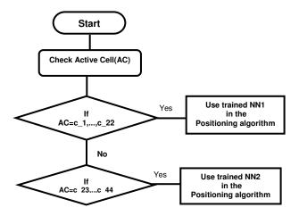
Figure 3: Flowchart showing the NN to be used in the positioning algorithm
