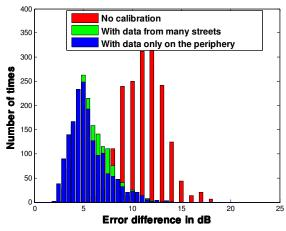
Figure 6: Histogram showing the dependence of calibration error on different scenarios
