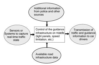
Figure 1 Functional architecture of a road traffic guidance system
