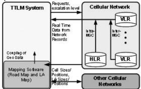
Figure 5 Server and communication architecture of the TTLM system
