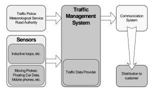
Figure 2 General structure of a traffic management system
