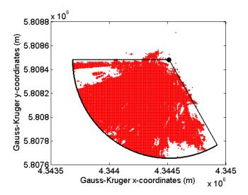
Fig. 2. For TA=0, the coverage area of a sector antenna as determined by the preprocessing step are illustrated (red spots) along with the borders of the area that would be considered when using only the antenna azimuth information (black arc and lines).
