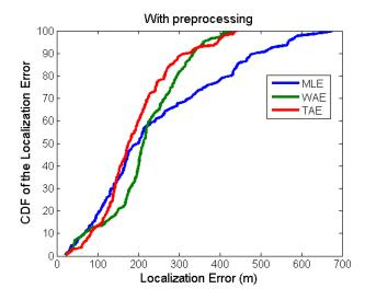
Fig. 3a. Cumulative distribution functions (CDF) of the localization error using the three methods of location estimation with preprocessing.
