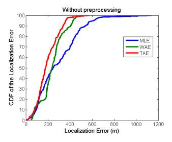
Fig. 3b. Cumulative distribution functions (CDF) of the localization error using the three methods of location estimation without preprocessing.
