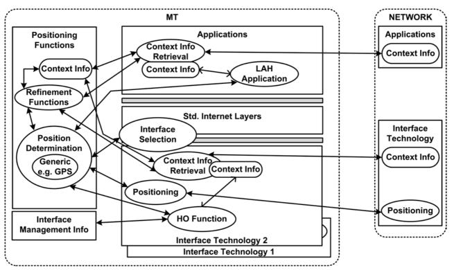
Figure 2. Multimode mobile terminal architecture for LAH
