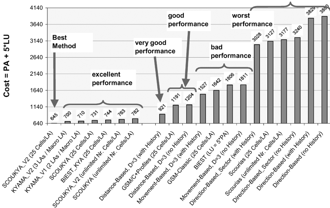
Fig. 20. Performance comparison of the different location management methods (average over CTM range 0 to 720)—average cost per day. (Simulation context: benchmark; geographical data of the town Hannover; average cell diameter 1000 m; user movements simulated over 60 days; D (in cells) is the threshold considered for the approaches distance-based and movement-based; location management cost = PA + 5*LU.)
